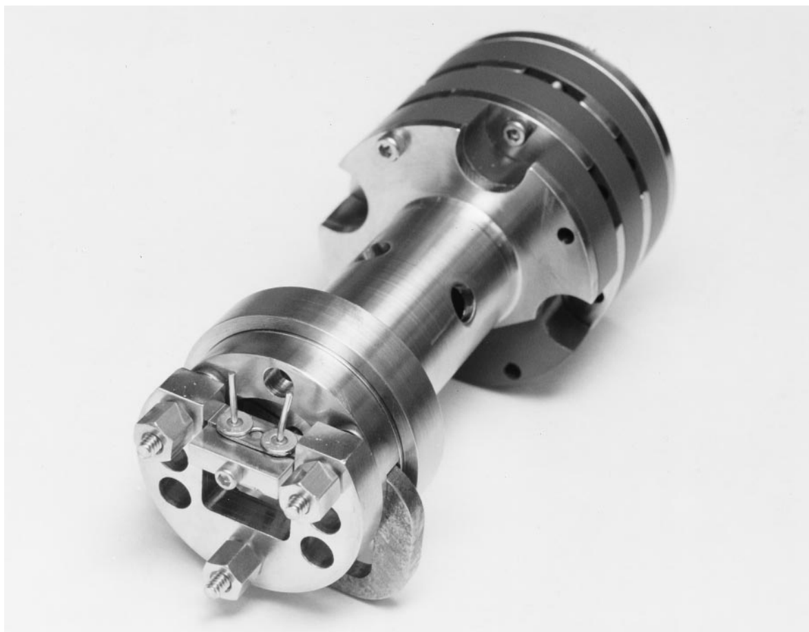
Fig. 4. As-built univoltage ion gun. Ion source gimbal assembly is at the left.
