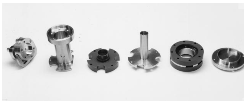
Fig. 5. Partially disassembled components of the univoltage gun.
